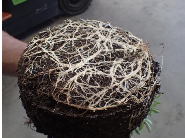
Photo 4 Root penetration through the bitumen layer of the reference specimen.
